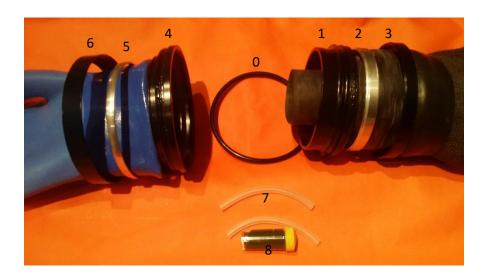
Coat the threads of parts n°1 and n°3 as well as n°6 and n°4 with the TED'S marine grade grease (n°8). Rotate back and forth to leave an even coat on the threads.
